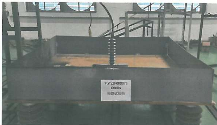
3 # Arrester before short-circuit test (6000A)
