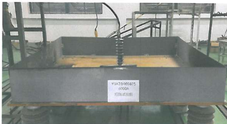
3 # Arrester after short-circuit test (6000A)
