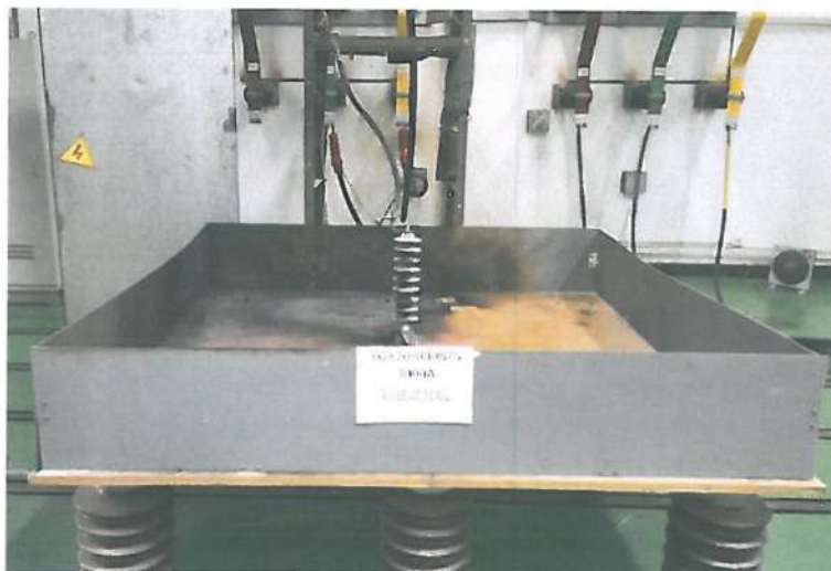
4 # Arrester after short-circuit test (3000A)
