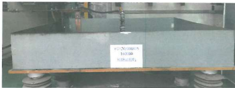
2 # Arrester after short-circuit test (16000A)
