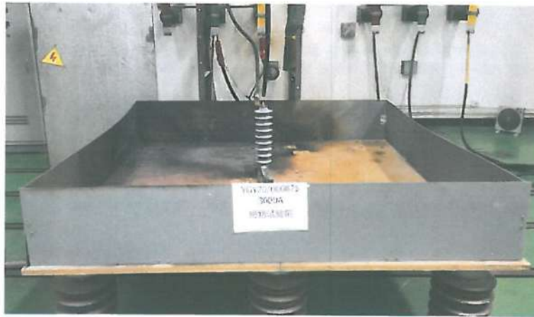
4 # Arrester before short-circuit test (3000A)
